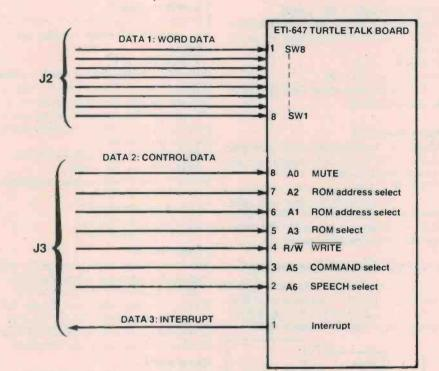
Figure 7. The synthesiser Interfaced via J2 and J3, showing the role of each line.
