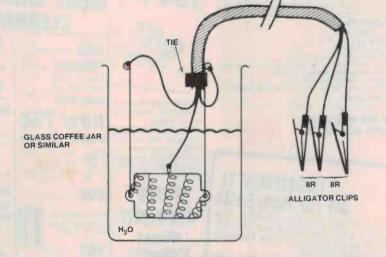
wires to the ends of the brass rods as shown in the diagram. Fit alligator clips or plugs to the other ends of this lead.
