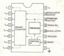
Figure 1. Functional block diagram of the XR-2240.
