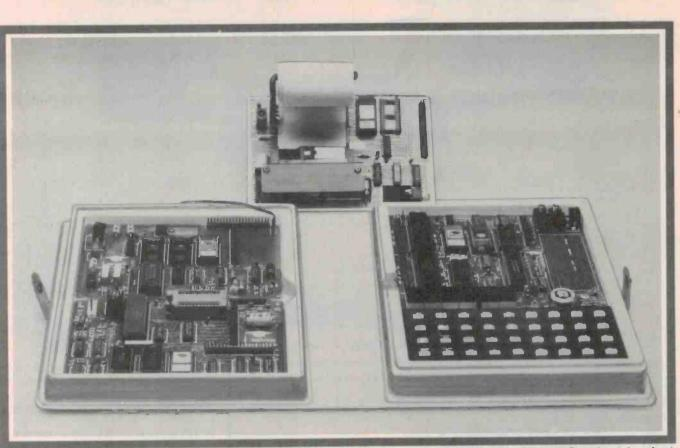
The 'full kit & kaboodle' Micro-Professor system. On the right, is the MPF-1, on PRT-MPF printer the left are the EPB-MPF EPROM programmer (foreground) and SSB-MPF designed so th speech synthesiser (behind the EPROM programmer). Right at the rear is the accommodated.
