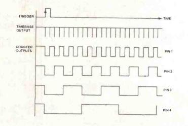
Figure 2. Output waveforms and timing diagram.
