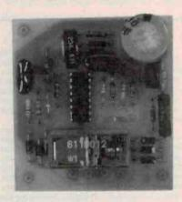
possible a truly 'set-and-forget' loudspeaker protector that can be mounted inside the loudspeaker enclosure if desired.
