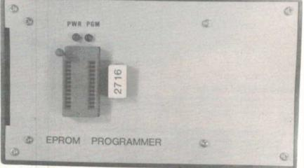
I housed the project in a jiffy box and lettered the front panel with Letraset. The 'ZIF' socket and 'personality' module DIP header are readily identified here.
