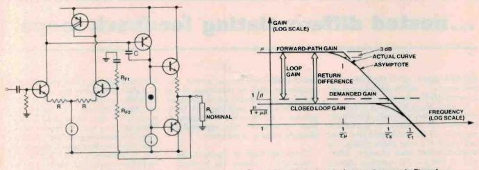
Figure 2. Outline circuit of an audio power amplifier.
