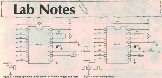
Figure 5. Astable operation under control of external trigger and reset controls.
