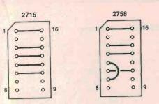
Figure 1 (left). Strapping of the personality module for 2716 programming.
